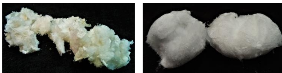
Fig. 1. (left) CA sample isolated without a step of deproteinization. It is slightly beige, and forms flakes (right) Deproteinized CA sample. It is white and fibrous, cotton-like
